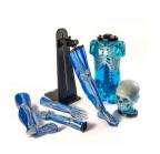
An ideal addition to any imaging department or Radiologic Technology training program, the CIRS products can assist in the monitoring, training and improvement of parameters and protocols common to most pediatric imaging procedures. The phantom is designed to assist technical and clinical staff in the selection, monitoring, training and verification of scanning parameters common to most radiological procedures requiring fine anatomical details.
