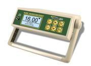
The AA-8000 is the latest in portable anesthetic agent analyzers. Utilizing proprietary state-of-the-art digital NDIR (Non-Dispersive Infrared) Technology it provides a low cost, high function, microprocessor-based analyzer that is simple to operate while maintaining high performance and accuracy.
